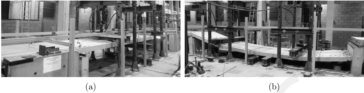
Figure 2: Global overview of the real-scale test set-up: original system 2a; after collapse 2b
