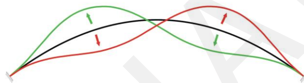
Figure 3. Second vibration mode.
