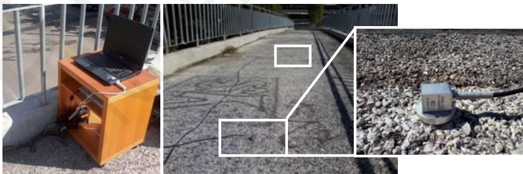
Figure 5. Wired data acquisition system applied on a small-scale academic instrumentation of a pedestrian bridge in Thessaloniki, Greece (Manolis et al., 2014)
