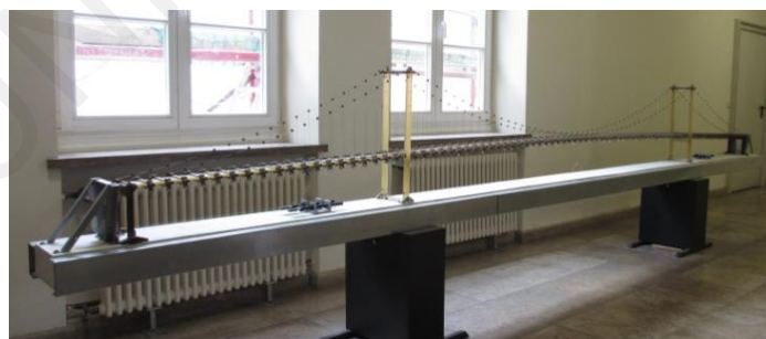
Figure 11. Laboratory model of the New Little Belt Bridge
