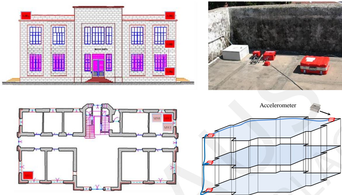
Figure 3. The 4 tri-axial strong-motion recorders used in the building [Genes et al. , 2012].
