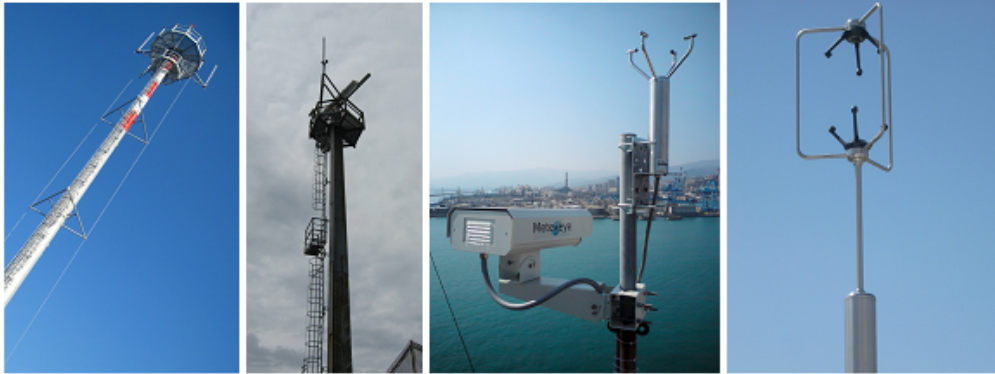
Figure 5: Wind monitoring network: three-axial and bi-axial ultrasonic anemometers
