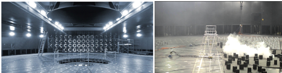
Figure 9: Inner chamber of the WindEEE Dome and a simulated downburst, (courtesy University of Western Ontario)
