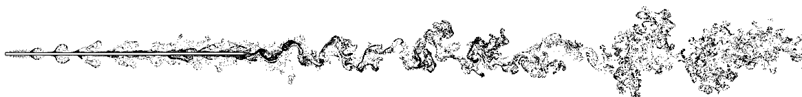
Figure 6.9: Forced vibration simulation on a flat plate (aspect ratio 100): instantaneous vortex pattern.
